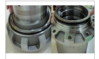
(17) Disassemble angular bearing (617).
