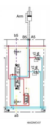
When the pilot pressure is led to the port a5, the oil from the pump flows to the cylinder port A5 and oil from the cylinder flows partially into the tank and partially trough regeneration path B to A through the cylinder port B5.
