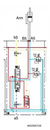
When the pilot pressure is led to the port b5, the oil from the pump flows to the cylinder port B5 and oil from the cylinder flows into the tank through the cylinder port A5.
