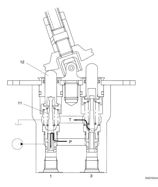
When the push rod (12) is stroked, the spool (11) moves downwards.
