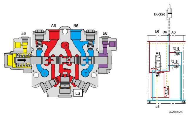
When the pilot pressure is led to the port a6, the oil from the pump flows to the cylinder port A6 and oil from the cylinder flows into the tank through the cylinder port B6.
