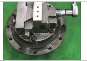
(5) Disassemble the spring cap (510)  $\rightarrow$  cap (509).
