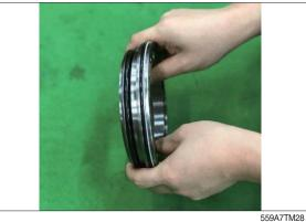
(20) The brake piston (114) is tapped lightly via the brake piston press jig and pressed into casing (202).
