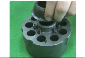
(13) Disassemble friction plate (118) and separator plate (119) in casing (202).
