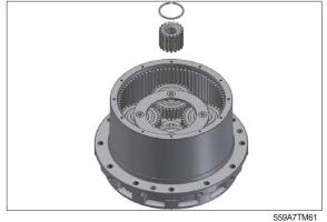
(9) Disassemble the No.2 holder assy.
