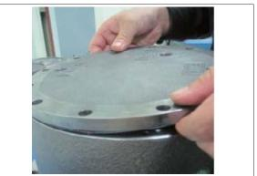
\* Be careful not to damage the O-ring (619) of the cover during disassembly.
