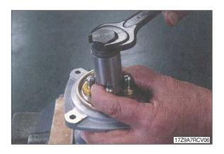
(6) Remove the plate (151).When the return spring (221) is strong
