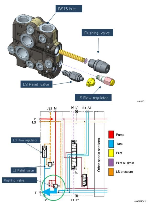
The Inlet element allows the exchange of the in the flow from the pump and the out flow to the tank.
