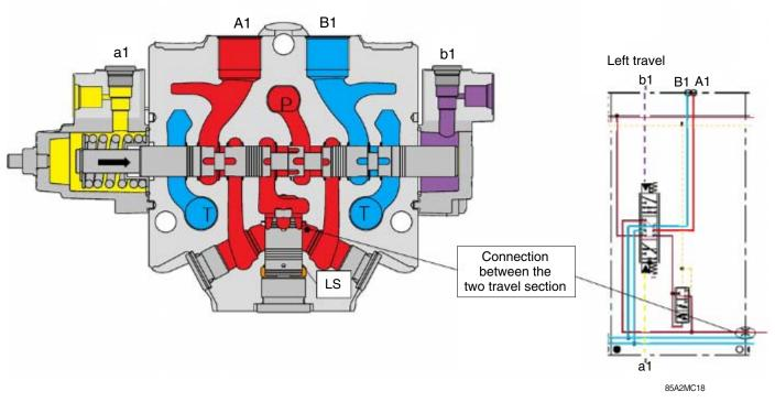
When the pilot pressure is led to the port a1, the oil from the pump flows to the cylinder port A1 and oil from the cylinder flows into the tank through the cylinder port B1.
