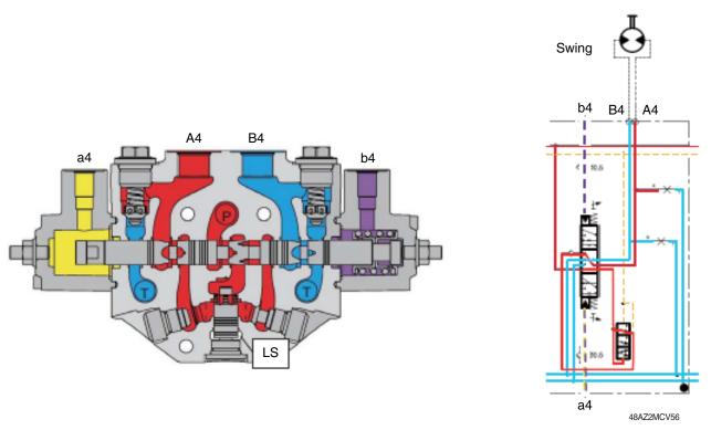
When the pilot pressure is led to the port a4, the oil from the pump flows to the motor port A4 and oil from the cylinder flows into the tank through the motor B4.
