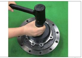
\* Pay attention to the assembly direction of the brake piston. The orifice of the brake piston is located downward on the same vertical line as the flow hole in casing.
