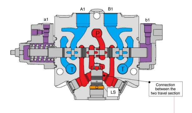
The spool is in neutral position, pump is in low pressure stand-by. The A and B ports are not connected to the pumps but to the tank. This is in order to ensure A and B to be drained to tank. The two translation branches, 1 and 2, are connected in order not to have differences in traction.
