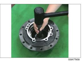
(12) Assemble pivot pin (113), pivot (112) to casing (202).
