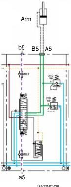
The spool is in neutral position, oil from the pump is blocked, pump is in low pressure stand-by. The A5 and B4 ports are not connected to the pump nor the tank.
