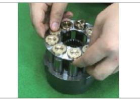
(18) Place casing (202) with the valve casing (201) assembly surface of casing (202) facing up. Separator plate (119) and friction plate
