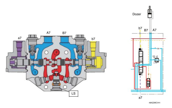
When the pilot pressure is led to the port b6 to maximal pressure, the spool is in the forth position, floating. The pump is in low pressure stand-by while A7 and B7 are connected to tank.
