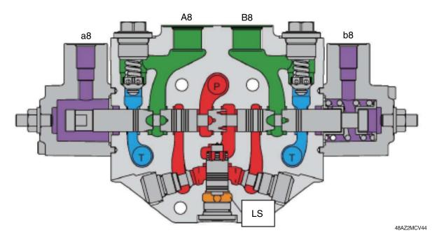
The spool is in neutral position, pump is in low pressure stand-by. The A8 and B8 ports are not connected to the pumps nor the tank.
