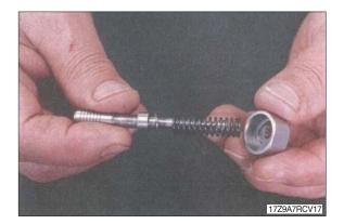
(2) Press down the spring seat (216) to flex the secondary pressure spring (241) while sliding the spring sideways through the larger aperture to attach it to the spool (201).
