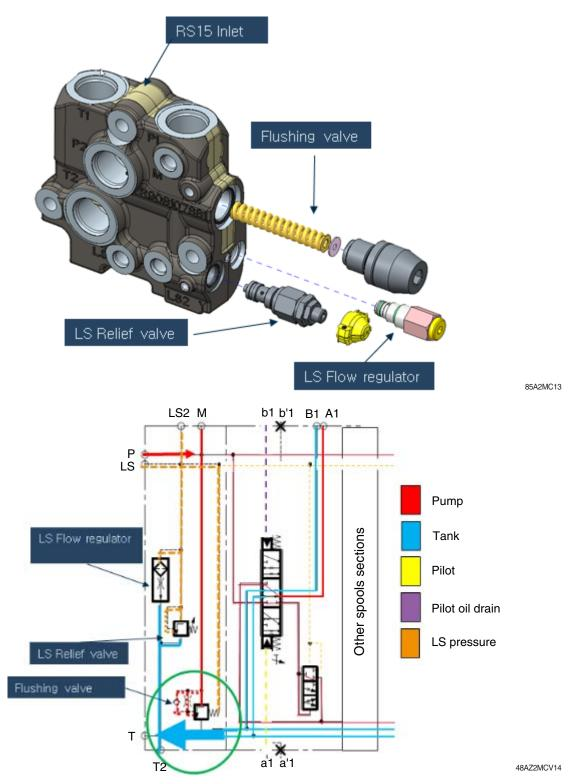
As soon as one or more spool moves, the flow stop to pass trough the flushing valve, which is closed, not anymore connected to the tank. The flow pass trough the spool to reach the movement, and then go to the tank by the T line after the spool.
