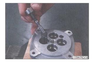
(4) Fit the O-ring (214) into the plug (221).
