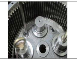
\* Caulking is performed to prevent loosening around the assembly.
