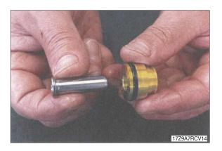
(12) Detach the O-ring (214) and seal (213)from the plug (211). Detach the seal (213) using a small screwdriver.
