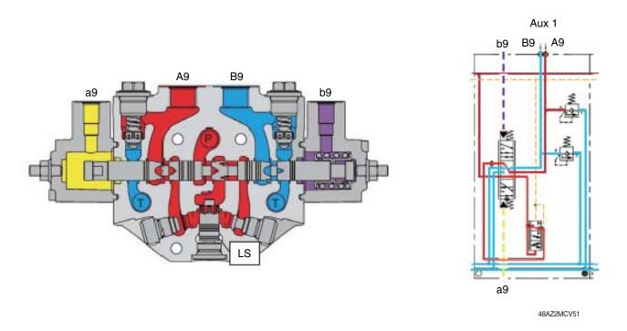
When the pilot pressure is led to the port a9, the oil from the pump flows to the cylinder port A9 and oil from the cylinder flows into the tank through the cylinder port B9.
