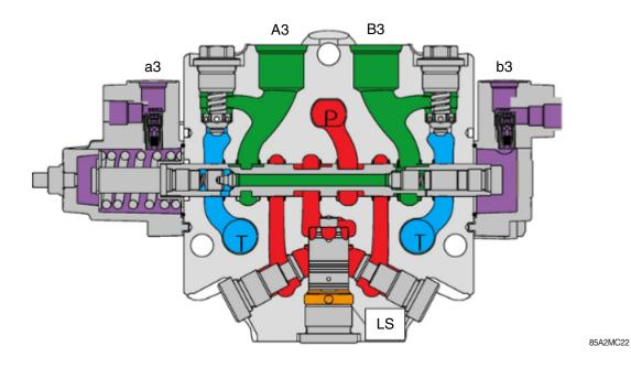
The spool is in neutral position, oil from the pump is blocked, pump is in low pressure stand-by. The A and B ports are not connected to the pump nor the tank.
